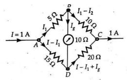
Q55. For the circuit given below, find the potential difference b/w points B and D.
