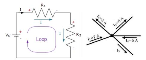
The directed sum of the potential differences (voltages) around any closed loop is zero.
