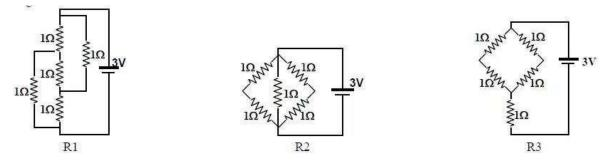
If the power dissipated by the configuration  $R_1$ ,  $R_2$  and  $R_3$  is  $P_1$ ,  $P_2$  and  $P_3$ , respectively, then (a)  $P_1 > P_2 > P_3$  (b)  $P_1 > P_3 > P_2$  (c)  $P_2 > P_1 > P_3$  (d)  $P_3 > P_2 > P_1$
